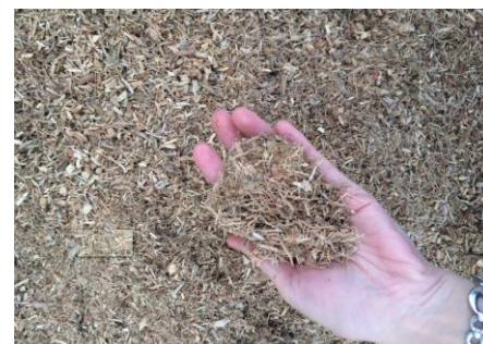
Coarse sawdust acting as bulking agent
