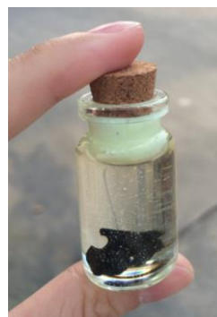
The black pieces are the slag remaining after plasma treatment.
